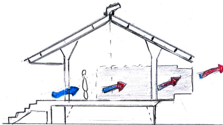
**Figure 1:** Parallel Openings effect on Cross-Ventilation System
