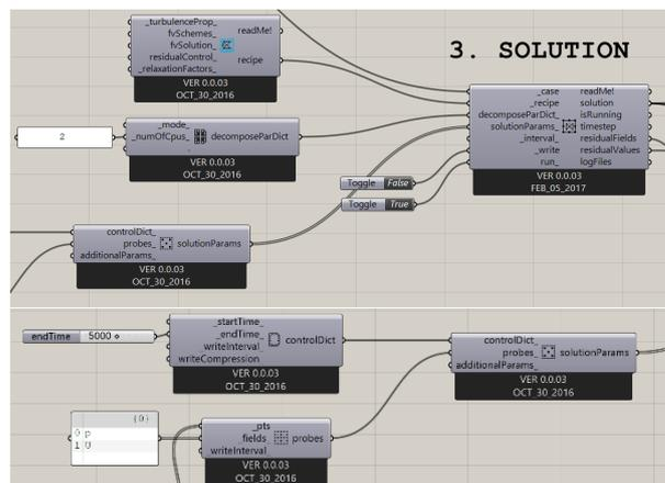
Figure 7 & 8: Creating solution code based on geographic location and adding wind velocity.
